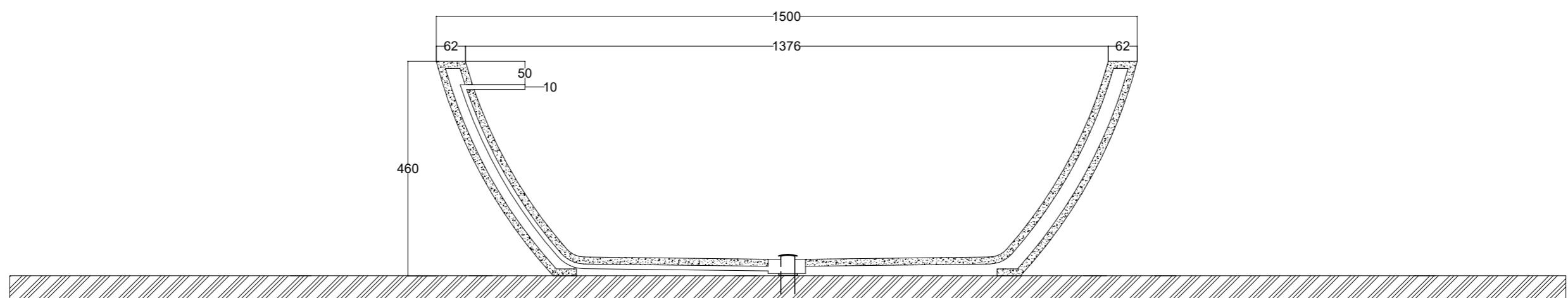
TB 14 Round Viet East, Size : 1500 x 1500 x 460 rim 62 mm With built in overflow line
